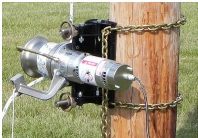
Rope lock device installed
