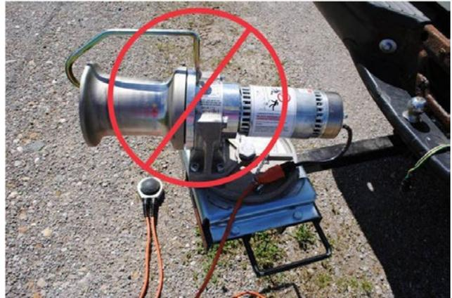
This Capstan hoist is incorrectly mounted. The drum should be over the swivel base.
