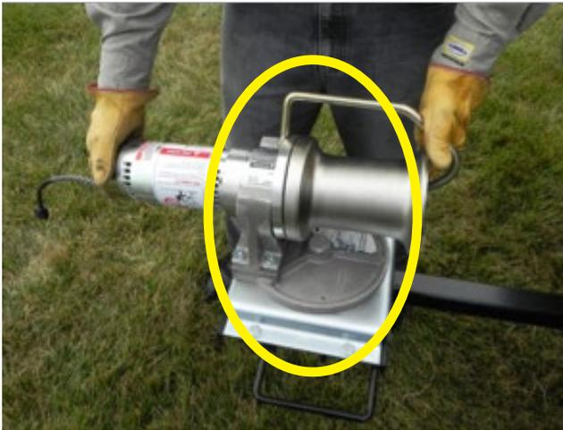
For a truck mounted swivel bracket application, the Capstan drum must be oriented so that the load line will be centered over the bolt that allows the mounting base to swivel. Incorrect mounting orientations will increase the load on the swivel base and may lead to equipment failure.
